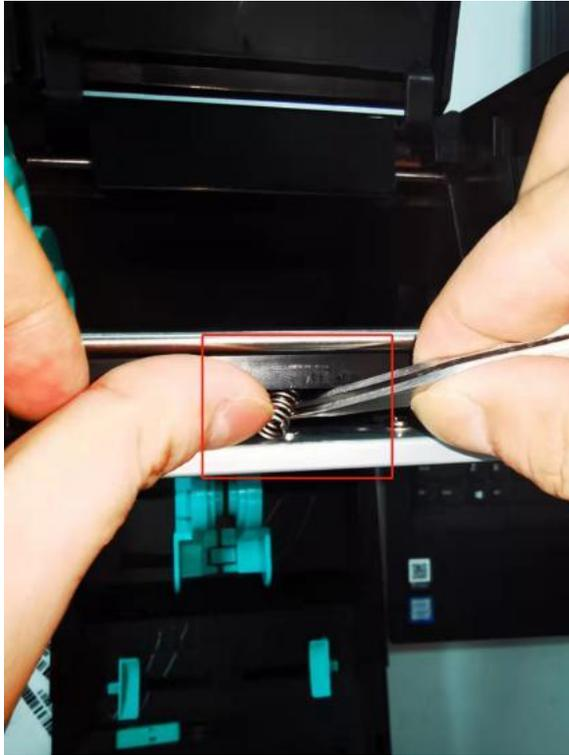
13. Install the other two screws to the spring in the same way.
