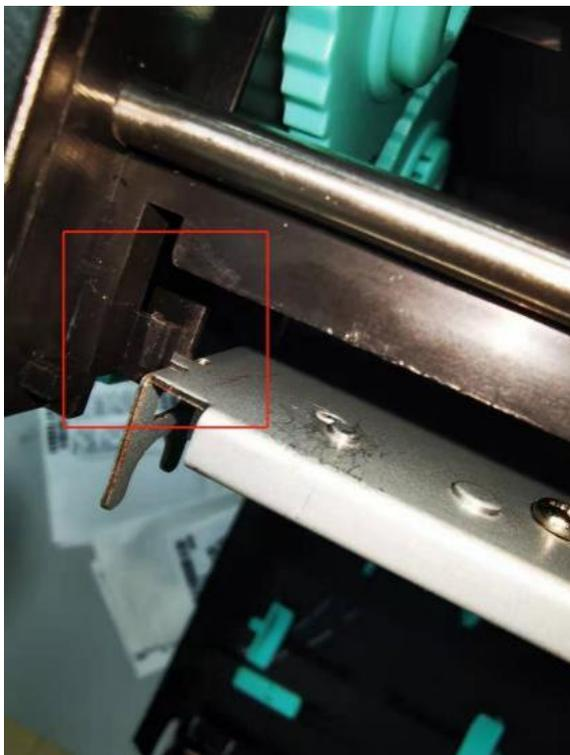
12. Hold the spring with tweezers (up to two laps) first, put the spring in the upper end of the printer, and then put the hand or tweezers in the buckle below:
