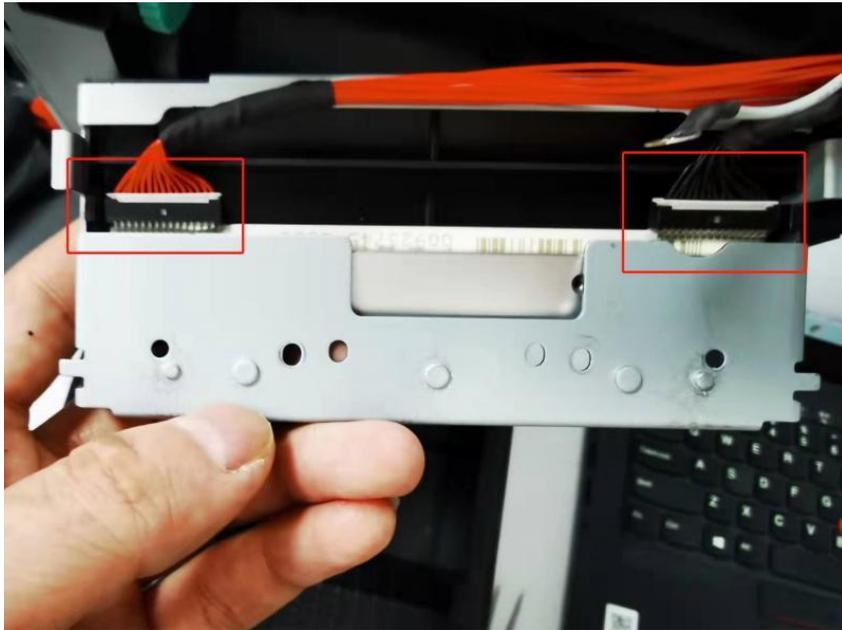
7. Install the print head : put the print head in the thermal bracket, pay attention to the front and back of the print head, and connect the print head online:
