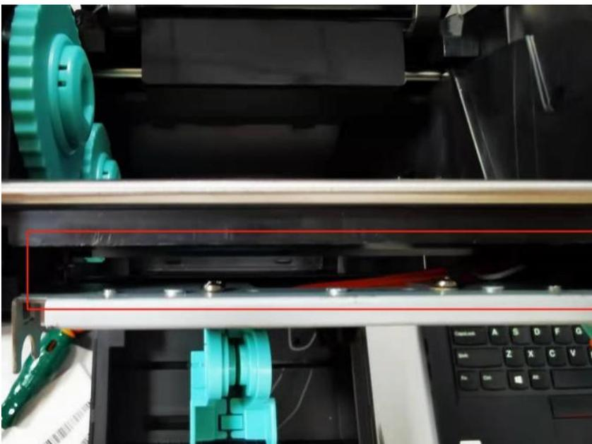
4. Press the pointing arrow and remove the print head.
