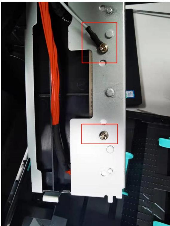
10.The thermal support shall be stuck in place:
